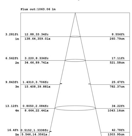
Height Eavg, Emax Angle: 105.03deg Diameter
